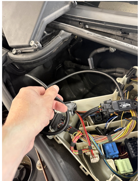
Route suitable vacuum hose from the MAP sensor to the selected inlet-manifold take-off.
