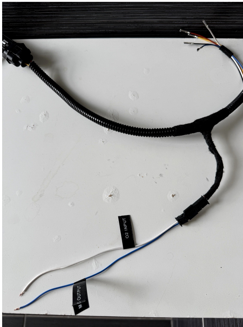
Optional tails are labelled on the harness: white = O2 INPUT; blue = MAC OUTPUT.
