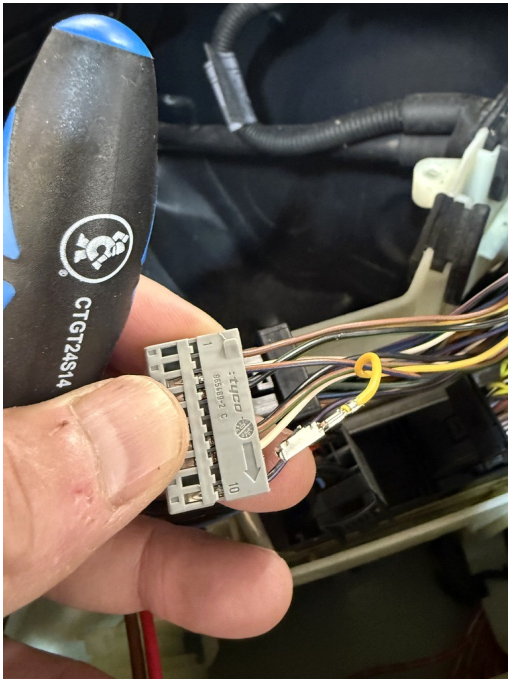
Close-up of the X60004 grey carrier during repinning.
